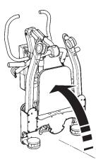
**NOTE:** If you wish to separate the mast and boom completely from the base and legs, undo the mast-locking lever fully (remove pin assembly from mast) and lift the mast and boom completely free from the base. Be careful not to lose the mast lock lever and location spindle.
