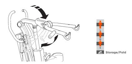
2. 2. Ensure the rear castors are securely locked (1). Raise the knee pad to its upper most position (2).
