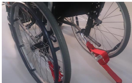
Fitting the Rear Restraint
