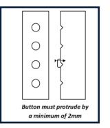
Some equipment items feature multi-hole adjustments on the legs which facilitates a minimal setting to compensate for uneven floor covering.
